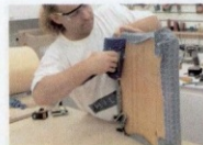
Start at center of each edge and pull fabric as tight as you staple
