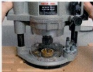
Rout vent holes using template and template guides
