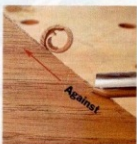
Digging in against grain
