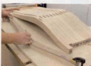
Use the template to locate the inside mortise (top and centre).
