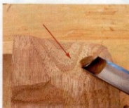
Grain line moves opposite to cutting direction
